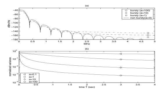
Fig. 2. Figure (a) compares the original 2B1Q HDSL disturber's PSD with the modified disturber's PSD for  $p_1 = 0.5$  and a = 0.1, 1, 10, 100. Figure (b) depicts  $(\sigma_h^2/p_1)$  as a function of T for different a.
