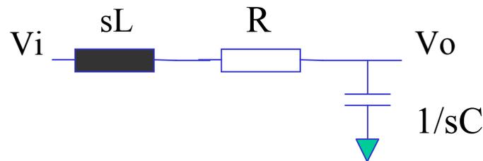
$$\begin{aligned} \frac{V_o(s)}{V_i(s)} &= \frac{Z_C}{Z_L + Z_R + Z_C} = \frac{1/sC}{sL + R + 1/sC} \\ &= \frac{1}{s^2 LC + sRC + 1} \end{aligned} \quad (1.30)$$
