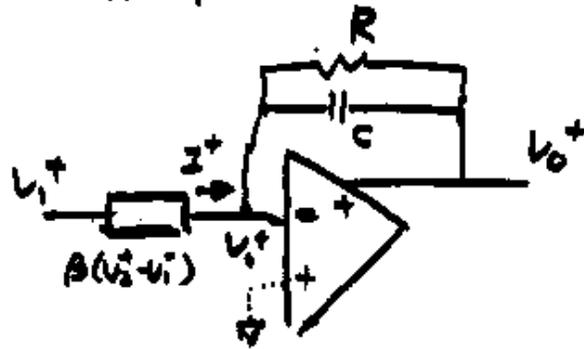
$$\begin{aligned} \underline{v_o^+ - v_o^-} &= -\beta [v_o^+ - v_o^-] [v_i^+ - v_i^-] [R \parallel \frac{1}{sC}] \\ &= -\beta (v_o^+ - v_o^-) (v_i^+ - v_i^-) \frac{1}{\frac{1}{R} + s} \end{aligned}$$
