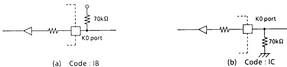
Figure 2. I/O code and external circuitry
