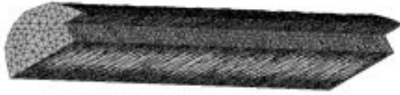
Figure 6. FEM mesh of one half of the keyed shaft workpiece.
