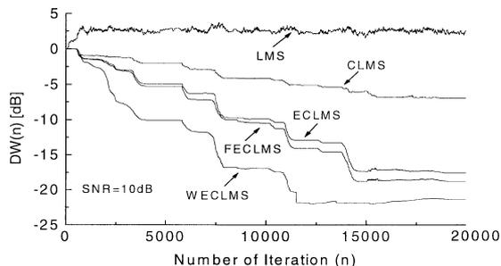
**Fig. 8** Comparison between LMS, CLMS, ECLMS, FECLMS and WECLMS in noisy double-talk condition.
