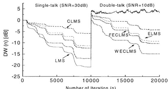
**Fig. 10** Switching from single to double talk with the echo path changed.
