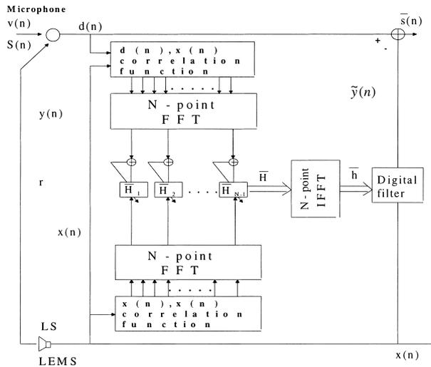
Fig. 3 Echo canceller by using FECLMS algorithm.
