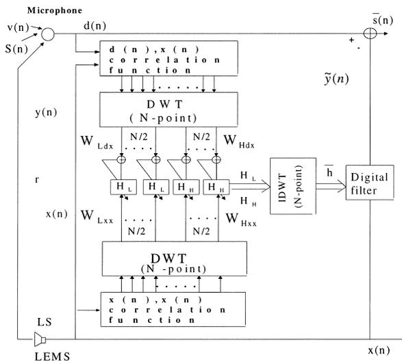
Fig. 4 Echo canceller by using WECLMS algorithm.
