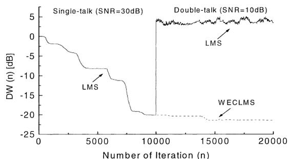
**Fig. 11** Switching from single to double talk with the same echo path by using the different algorithm.
