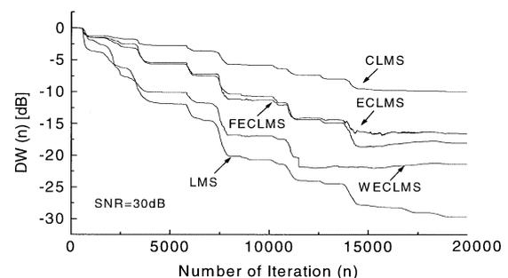
**Fig. 7** Comparison between LMS, CLMS, ECLMS, FECLMS and WECLMS in noisy single-talk condition.
