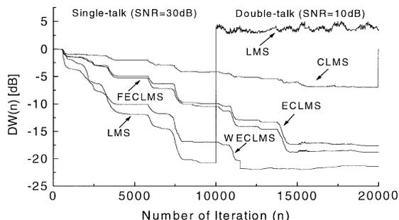
**Fig. 9** Switching from single to double talk with the same echo path.
