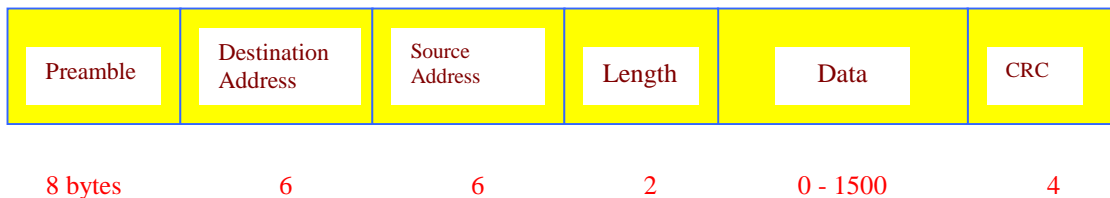
Figure (2-1) Ethernet Frame
