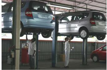
PDI Center or Pre-Delivery Inspection Center is where the cars are checked and ready for delivery to dealer.
