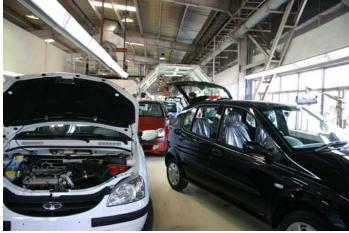
When the vehicles first rolled out from the factory, it will be move to an inspection area to inspect the vehicles road readiness. Once passed, the vehicle will be sent out from the factory.
