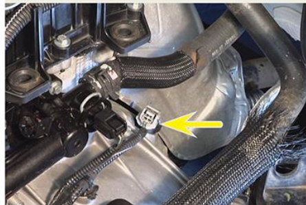
Fig.18 - Sensor CKP instalado
