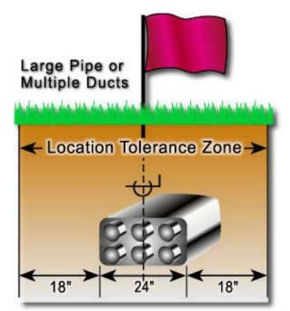
The width of the tolerance zone is specified in the law. The tolerance zone includes the width of the facility and 0.5 m (18") measured horizontally from each side of the facility.
