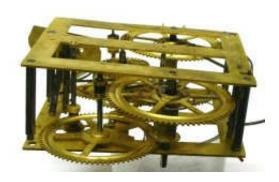
After you assemble the mechanism, you want to check the relationship between the gears in the strike train. At the moment the stop lever (known formally as the detent) enters the slot in the cam,
