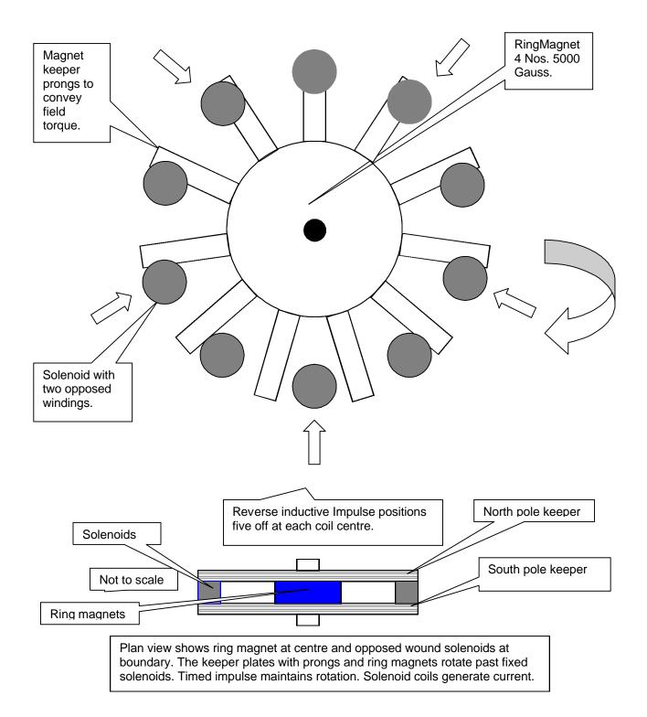
Direction of motion Of Magnetic rotor Eleven prongs positions shown
