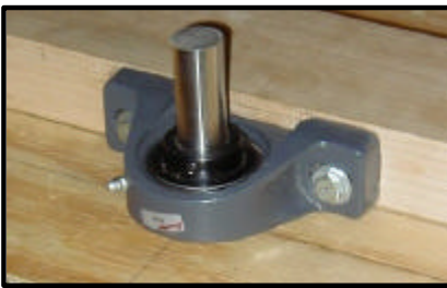
Upper bearing is bolted to hardwood 2 x 4 that is bolted to top-side braces. Turning wheel can be plywood or purchased metal one.
