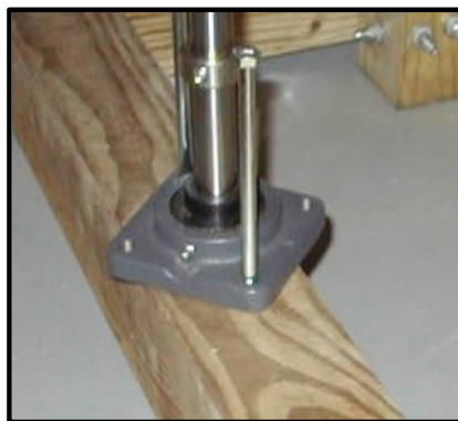
Bottom bearing is flange-type, I should have used a 2 hole. "Oh Well." A recess is made in 4x4 support for the rod end.
