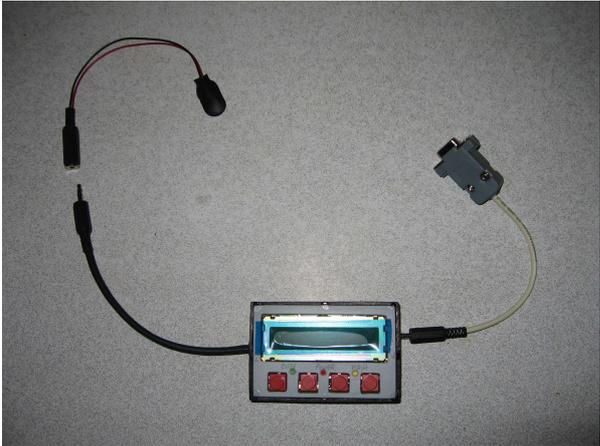
Cable connection for serial terminal and
