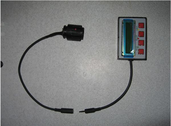
Cable connections for C1 diagnostic mode
