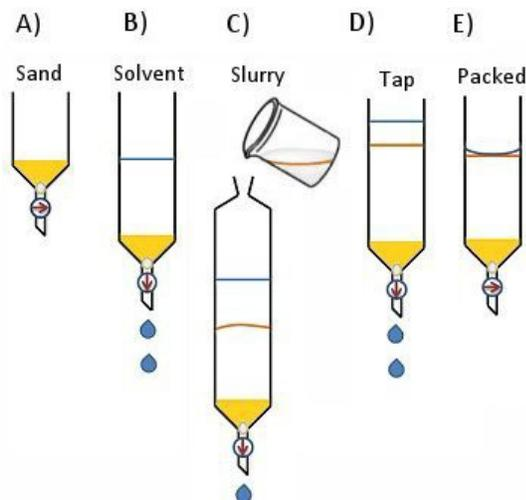
**Top Tip:** Use hand bellows to increase the pressure in the column and to force the silica to compact. Repeat several times, rinsing the sides of the column in between, to ensure complete packing.
