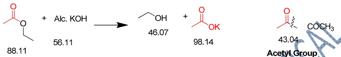
A weighed amount of the ester is heated with a known volume (excess) of the standard alkali hydroxide solution and the excess of alkali is determined, after hydrolysis is complete, by titration with standard acid.
