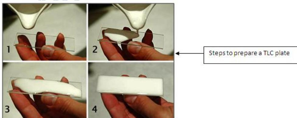
Developing TLC plates using SiO<sub>2</sub> on Glass /Aluminium plate
