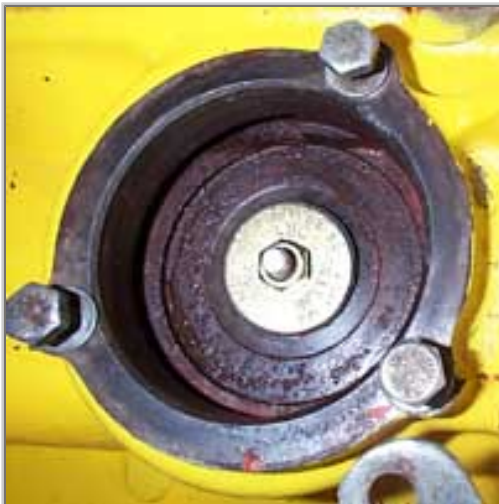
The upper cavity sealed with the expandable rubber freeze plug.
