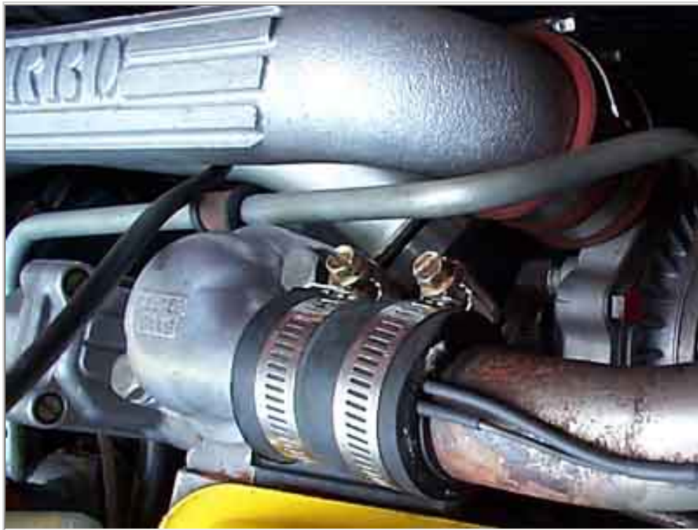
The wiring for the sensor passes through the upper hose by means of an adapter supplied with the EWP Controller.
