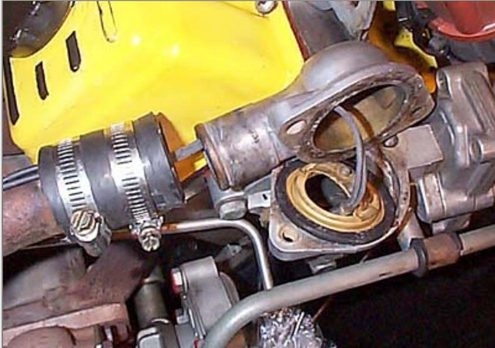
The EWP sensor wiring is shown here passing through the thermostat, housing cover and through the radiator hose using the adapter supplied with the EWP Controller. The sensor rests inside the thermostat cover.
