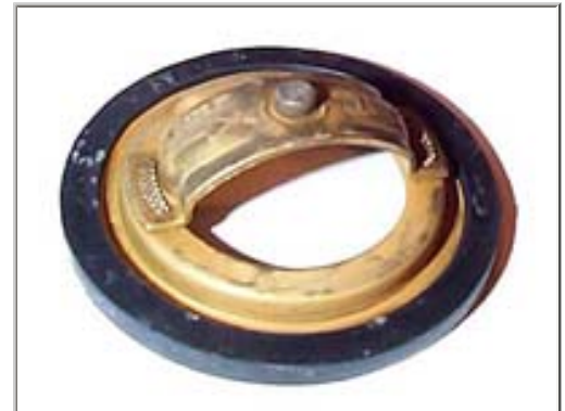
The stock thermostat with its center section removed, ready to be reinstalled.
