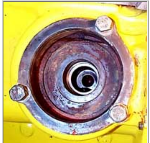
The water pump cavity after removal of the original waterpump.
