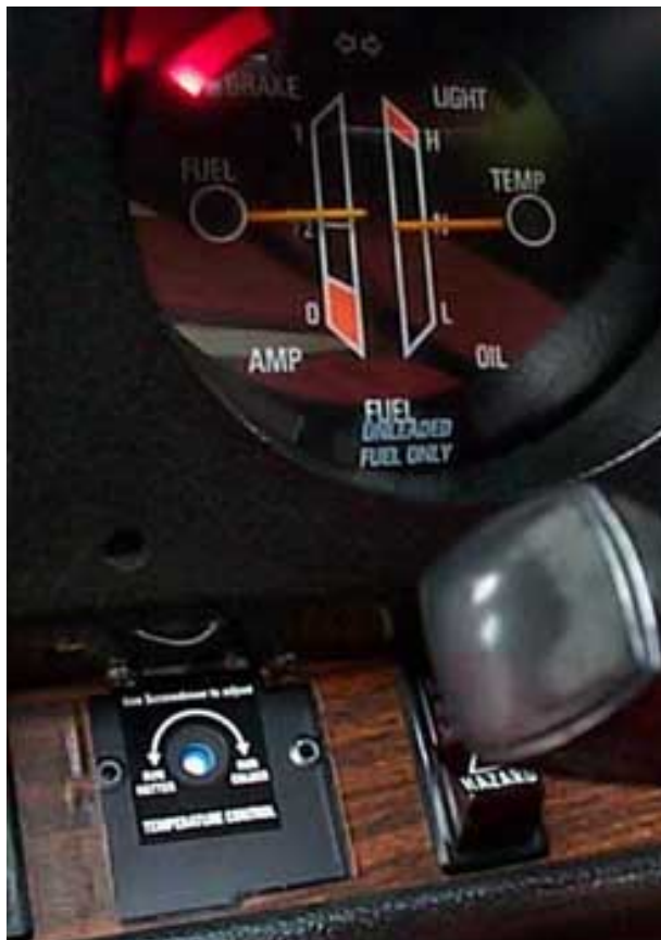
A stock look can be achieved by installing the Controller behind some of the extra switch panels on the 99 dashboard.
