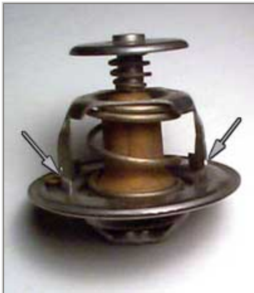
Cut the arms where indicated by arrows to remove the center section of the stock thermostat.
