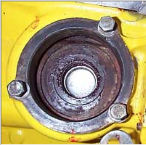
The lower cavity sealed with the metal freeze plug.
