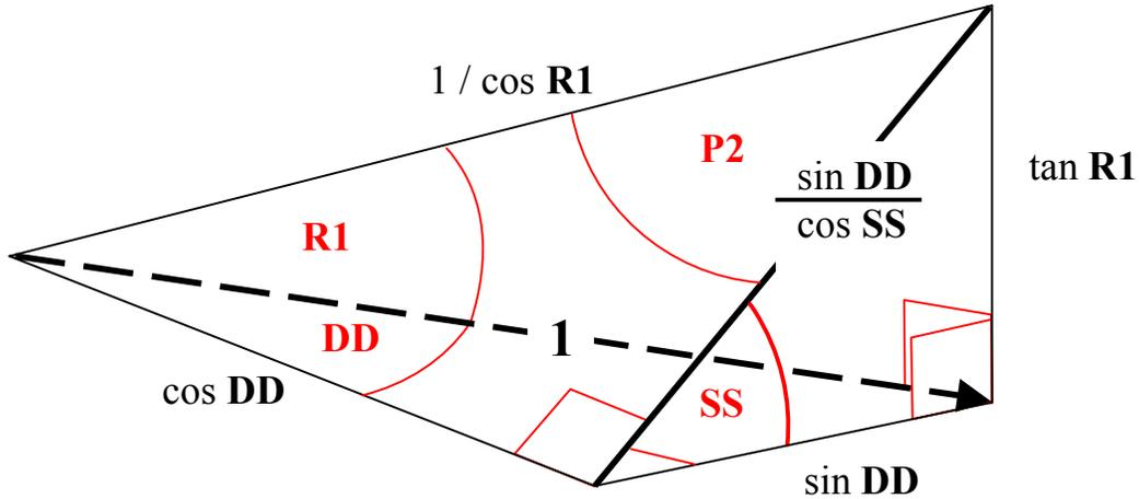
$$\begin{aligned} \tan P2 &= \frac{\cos DD}{(\sin DD / \cos SS)} \\ &= \cos DD \cos SS / \sin DD \\ &= \cos SS / \tan DD \end{aligned}$$
