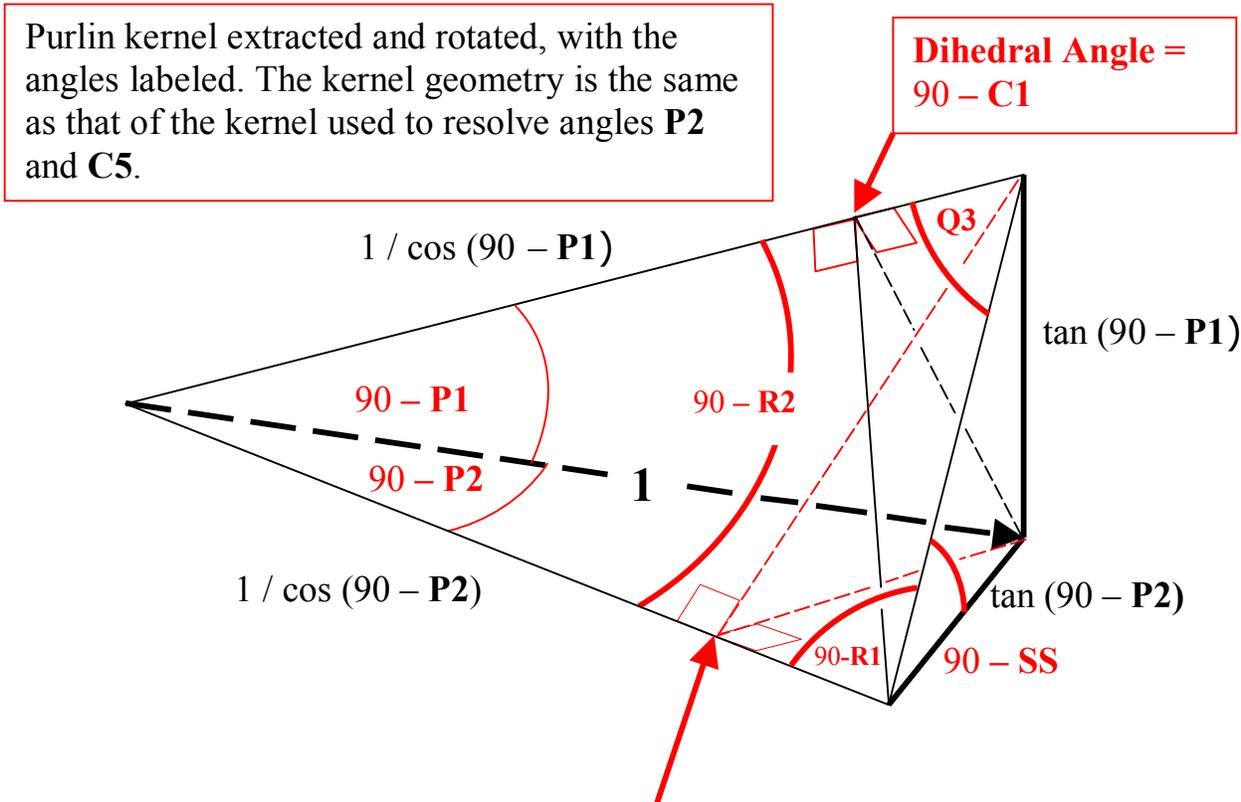
The kernel may be divided along the lines of dihedral angle  $90 - C5$ , resulting in two kernels: the kernel of Common rafter angles, and a kernel the same as that extracted from the stick. However, this kernel will be analyzed as it sits, to demonstrate that there is more than one method, or one type of geometry, whereby it is possible to obtain angle formulas.
