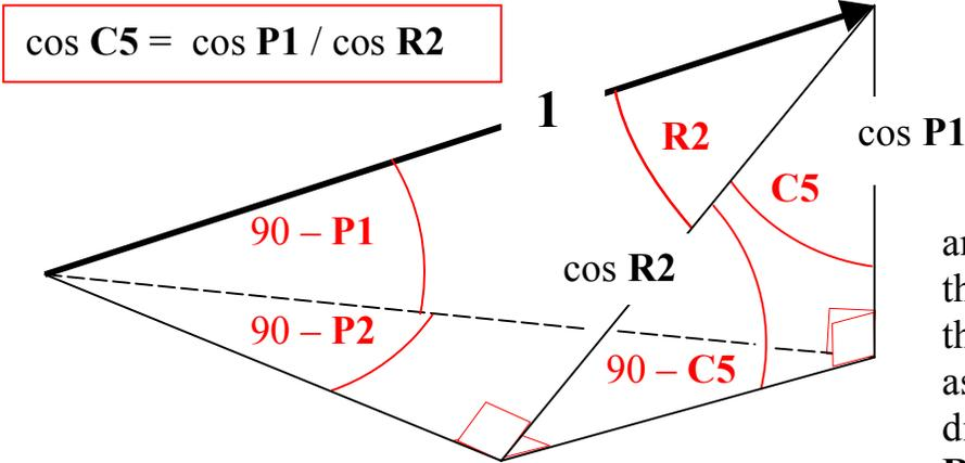
Compare this kernel, and the original diagram of the Purlin kernel situated on the Hip kernel. The line assigned the unit value in this diagram defined angle  $90 - R2$  in the original diagram (dashed line). In the sketch below, either of the lines may be used as a reference length.
