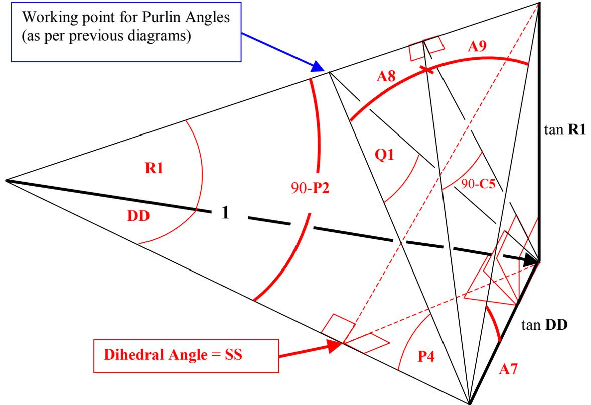
The same kernel geometry was required to solve backing angle C5, and the purlin related angles. Lines tan DD, tan R1, and the unit vector are mutually perpendicular. The planes of angles A7, C5, Q1 and DD are all perpendicular to the plane of Hip/Valley pitch angle R1; that is, all of the planes created are at right angles to the side face of the Hip/Valley.
