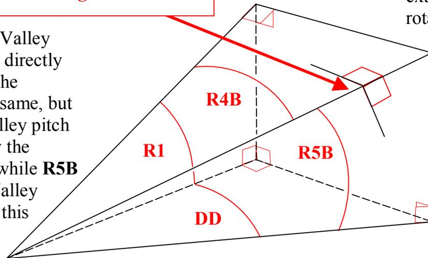
Kernel with the angles labeled. Remember that the standard model is a Hip kernel (refer to the diagram on the previous page). The angles located at the foot, or *base*, of a hip rafter will be found at the *peak* of a valley rafter.
