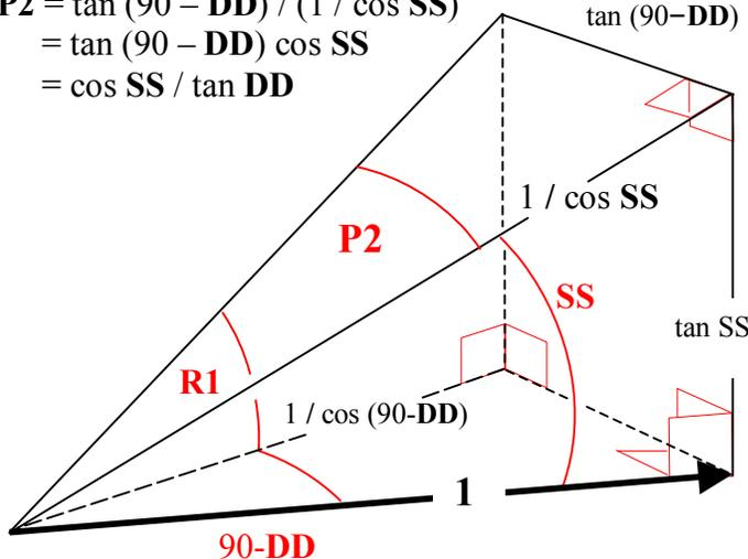
Observe that we have a general equation for the revolution of any angle, given this scenario. The tangent of the resulting angle on the cutting plane (**R1**, or **P2**, as the case may be) equals the tangent of the original dihedral angle multiplied by (the same as division by the reciprocal) the cosine of the angle of revolution.
