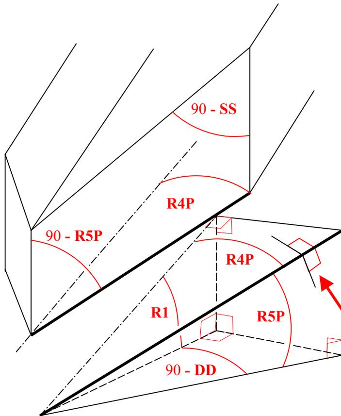
To calculate angles at the base or foot of a valley rafter, consider a kernel positioned below the rafter as shown in the diagram to the left. The “roof plane” of the kernel is parallel to the bottom shoulder of the valley rafter (imagine the rafter seated on the kernel).
