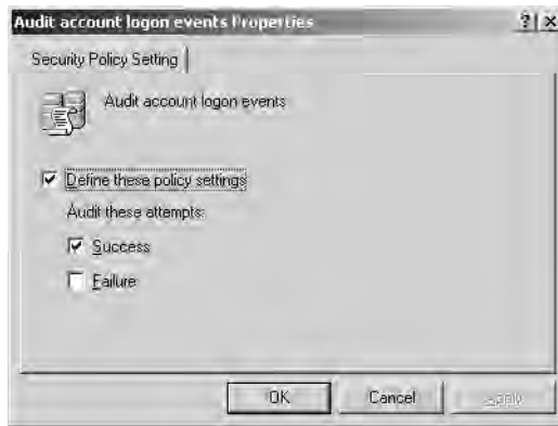
Figure 13-10 The Properties dialog box for the Audit Account Logon Events event category
