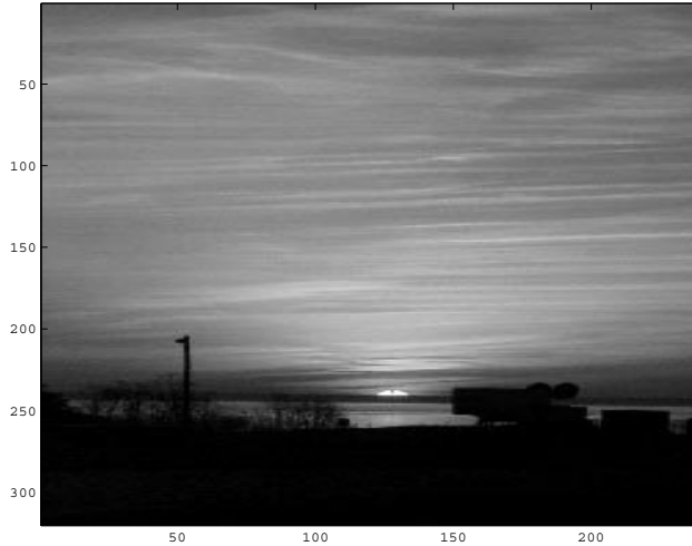
Figure 5.10 The result of mapping a 256-gray-level image to 64 gray levels using imagesc .
