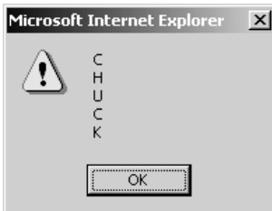
Figure 5-3. Each line displayed is a distinct argument handed to the createList() function.
