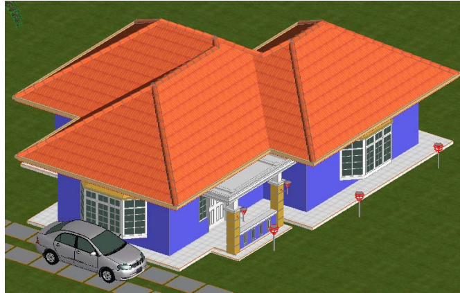
Gambar 1.4 Jenis proyeksi Isometric axonometry
